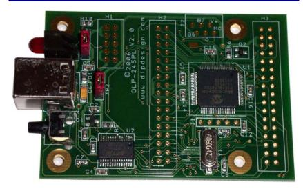
The DLP-245PL-G combines the same lead-free USB interface used in the DLP-USB245M-G module with a Microchip PIC microcontroller to form a rapid development tool. The 18LF8722 microcontroller is preprogrammed with basic functionality for accessing the port pins and can be reprogrammed with user hex code via a 5-pin header that is compatible with Microchip's MPLAB ICD2 device programmer/debugger (purchased separately).
